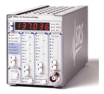
The SIM921 AC Resistance Bridge is a precision, low noise instrument designed for cryogenic thermometry applications. With achievable excitation power below 100 aW, thermistors and other resistive samples can be measured at temperatures below 50 mK with negligible self-heating errors.
